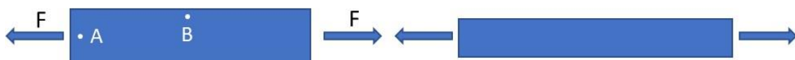
Figure 1: Deformation of a rectangular flat piece under forces applied at the narrow ends. Left: before deformation. Right: deformed piece.
